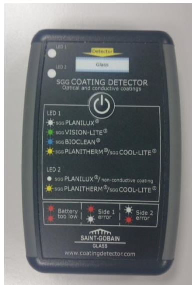
Figure 2: Example of adapted detector for BIOCLEAN® (II)
